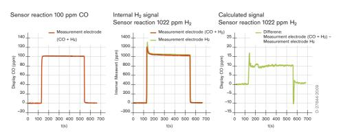
The values shown in the following table are standard and apply to new sensors. The values maybe fluctuate by  $\pm$  30%. The sensor may also be sensitive to additional gases (for more information, please contact Dräger). Gas mixtures may be displayed as the sum of all components. Gases with a negative cross sensitivity may displace an existing concentration of CO. To be sure, please check if gas mixtures are present.
