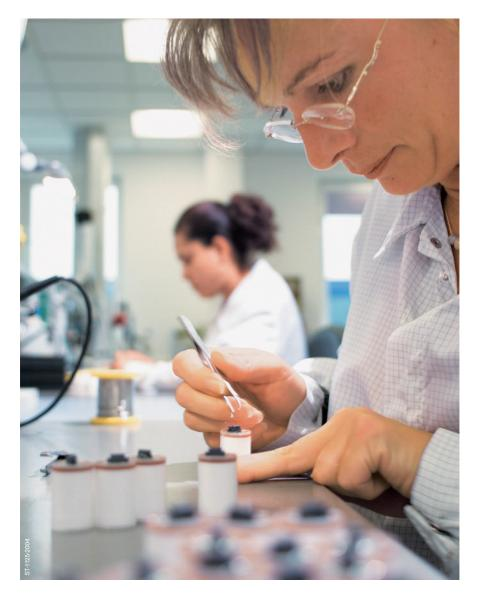
Many toxic gases are highly reactive and can change their chemical composition under certain conditions. An electrochemical sensor is a micro-reactor, which produces a very small but measurable current when reactive gases are present. As in a normal household battery, this involves an electrochemical process, since the chemical transformation produces electrons.
