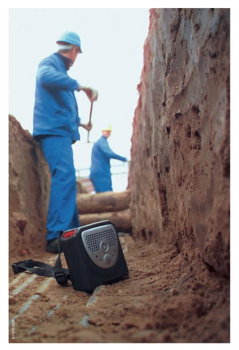
If hazardous substances (Ex-Ox-Tox) occur in the work place, then it is advisable to use continuous multi-gas measuring instruments. These enable different measuring approaches be used (infrared, catalytic bead, PID, and electrochemical sensors) in one device, thus drawing on the strengths of the measurement principles.
