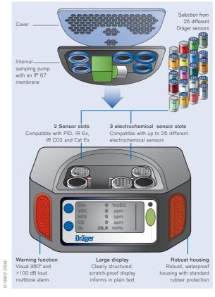
Gas measurement technology (example: Dräger X-am 7000)
