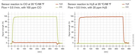
The values shown in the following table are standard and apply to new sensors. The values maybe fluctuate by  $\pm$  30%. The sensor may also be sensitive to additional gases (for more information, please contact Dräger). Gas mixtures may be displayed as the sum of all components. Gases with a negative cross sensitivity may displace an existing concentration of CO or H<sub>2</sub>S. To be sure, please check if gas mixtures are present.
