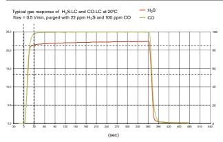
The values shown in the following table are standard and apply to new sensors. The values maybe fluctuate by  $\pm$  30%. The sensor may also be sensitive to additional gases (for more information, please contact Dräger). Gas mixtures may be displayed as the sum of all components. Gases with a negative cross sensitivity may displace an existing concentration of CO or H<sub>2</sub>S. To be sure, please check if gas mixtures are present.
