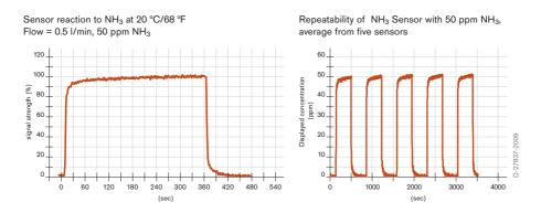
The values shown in the following table are standard and apply to new sensors. The values maybe fluctuate by  $\pm$  30%. The sensor may also be sensitive to additional gases (for more information, please contact Dräger). Gas mixtures may be displayed as the sum of all components. Gases with a negative cross sensitivity may displace an existing concentration of NH<sub>3</sub>. To be sure, please check if gas mixtures are present.
