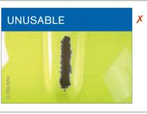
Helmets with extensive material abrasion reaching down to the black helmet shell material must be classified as unusable.
